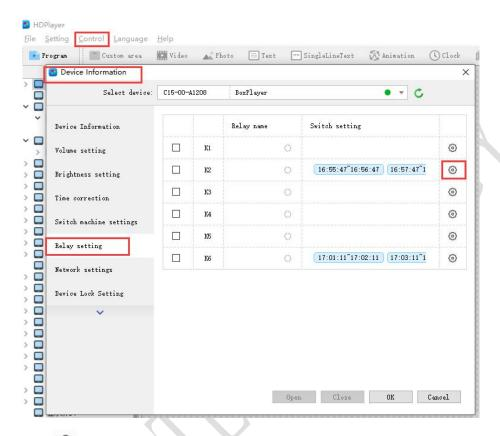
2.Click the setting button to enter the time setting interface and set the time for ports K1-K6.
